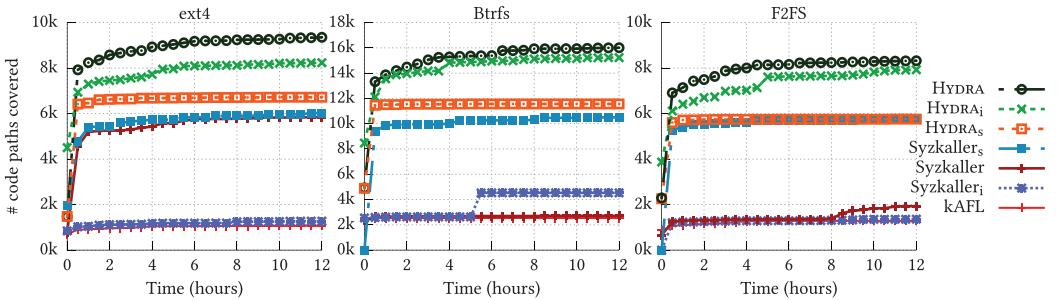
Fig. 16. Code coverage for 12 hours of fuzz testing with kAFL, Syzkaller, HYDRA, and their variants ( $i$  for image-only and  $s$  for syscall-only mutation). It indicates that HYDRA aggressively explores the input space that both kAFL and Syzkaller could not reach, and combining both image and input mutators exhibit a synergistic effect in exploring different parts of the input space.
