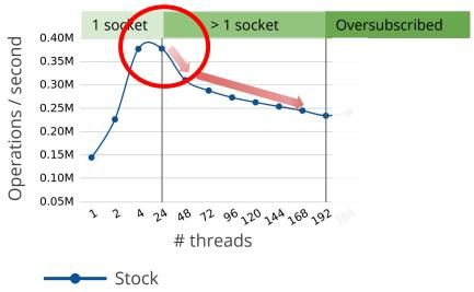
Setup: 192-core/8-socket machine
