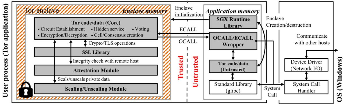
Fig. 1. The architecture of SGX-Tor. Gray-colored boxes indicate modified or newly added components from the original Tor. The address space of the Tor application is divided into: *enclave memory* and *application memory*. The enclave communicates only with untrusted software through a well-defined interface.
