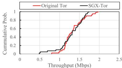
Fig. 7. Hidden service throughput of SGX-Tor and original Tor.
