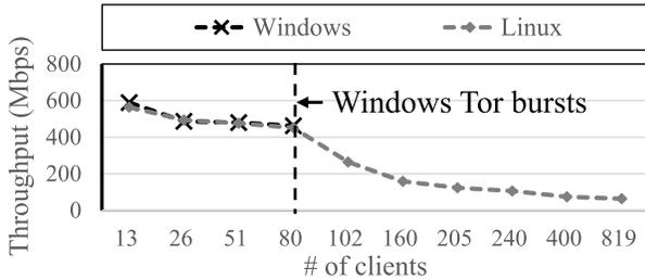
Fig. 12. Stress test of Linux and Windows SGX-Tor.
